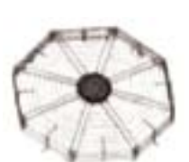
Octangular grill air flow resistance reduction
